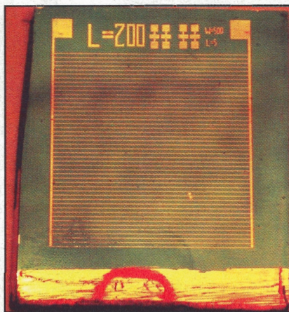
The organic field effect transistors were grid-electrode devices with dimensions of 10 \times 14 mm.
