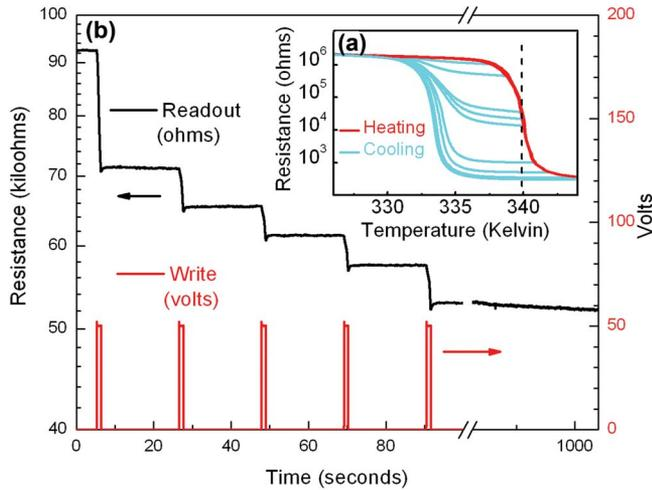
FIG. 2. (Color online) (a) Resistivity-temperature curves of our device illustrating the hysteretic nature of the IMT phase transition. The vertical dotted line shows the bias temperature for experiments of Figs. 1(b) and 2(b). (b) Demonstration of information storage in a memristive vanadium dioxide film. Each 50 V pulse triggers the transition to a new resistivity level.
