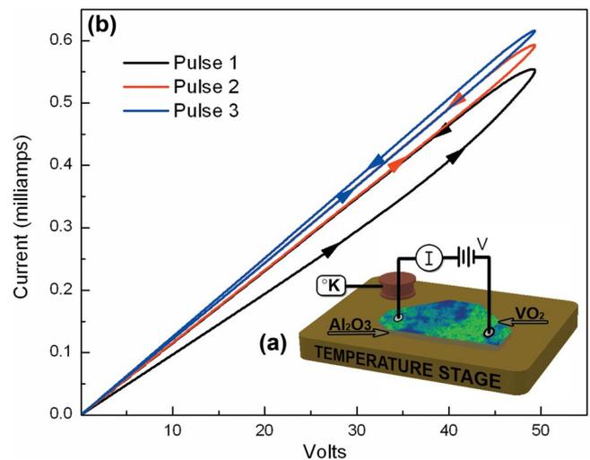
FIG. 1. (Color online) (a) Schematic of the device. The area of the VO<sub>2</sub> film is  $\sim 25$  mm<sup>2</sup>. (b) Three current-voltage (*I-V*) curves for our device exhibiting nonlinear hysteretic behavior which is indicative of a memristive system.
