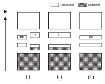
FIG. 6. Schematic energy level diagram displaying three possible scenarios for an insulator-metal transition in P3HT upon doping: (i) a first-order transition from a bipolaron to a polaron lattice, leading to a partially-filled band; the (ii) polaron or (iii) bipolaron band broadens to merge with the valence band.
