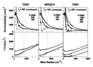
FIG. 2. The optical conductivity  $\sigma_1(\omega, T)$  and scattering rate  $1/\tau(\omega, T)$  for Tl2201 at doping levels with  $T_c = 90$  K (maximum) and  $T_c = 23$  K (strongly overdoped) and Bi/Pb2212 with  $T_c = 70$  K (overdoped). The spectra at T = 10 K are shown by the thin lines.
