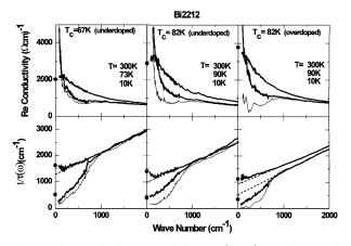
FIG. 1. The optical conductivity  $\sigma_1(\omega, T)$  and scattering rate  $1/\tau(\omega, T)$  for Bi2212 at several doping levels. The temperatures shown are room temperature, just above  $T_c$ , and well below  $T_c$  (thin lines). The straight dashed lines show a linear fit to  $1/\tau(\omega, T)$  over frequencies 800–3000 cm<sup>-1</sup>, while the dots show the results of dc measurements.
