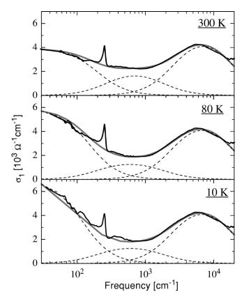
FIG. 3. Drude-Lorentz fits of the optical conductivity  $\sigma_1(\omega)$  at 300, 80, and 10 K. As temperature decreases, the Drude peak narrows, but its spectral weight appears to be conserved. The 7000-cm<sup>-1</sup> peak is only weakly temperature dependent.
