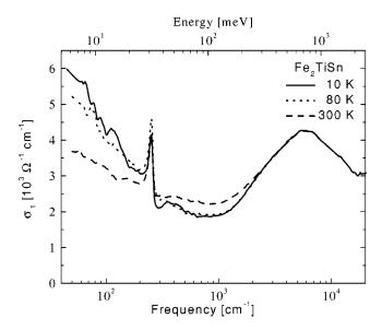
FIG. 2. The optical conductivity  $\sigma_1(\omega)$  of Fe<sub>2</sub>TiSn is characterized by a narrow Drude mode and an interband transition at around 7000 cm<sup>-1</sup>. A strong peak at 250 cm<sup>-1</sup> is an optically active phonon mode.
