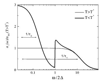
FIG. 4. Schematic behavior of the frequency-dependent optical conductivity  $\sigma_1(\omega)$  in an *f*-electron HF system. Note that below T\* both  $1/\tau$  and  $\omega_p$  of the Drude mode are strongly reduced.
