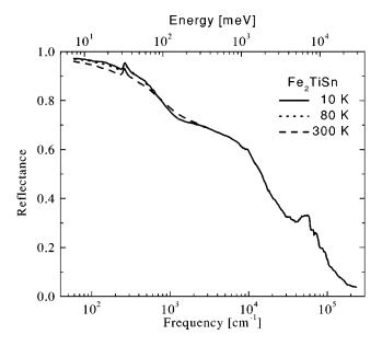
FIG. 1. The reflectance data of  $Fe_2TiSn$  at 10, 80, and 300 K. The spectra show anomalous temperature dependence in the midin-frared range.
