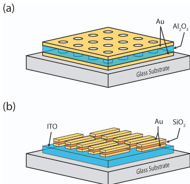
Fig. 10. Metamaterials used for response at near-IR and optical frequencies. (a) A schematic of the multilayer structure used in Ref. 36 consisting of an  $\text{Al}_2\text{O}_3$  dielectric layer between two Au films with a square array of holes (pitch of 838 nm, diameter of 360 nm). (b) Shows the pairs of Au nanorods used in Ref. 19 separated by a  $\text{SiO}_2$  layer on top of a glass substrate separated by a 180 nm layer of indium tin oxide (ITO).
