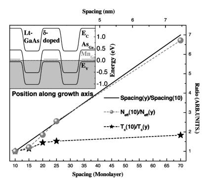
FIG. 4.  $N_{eff}^{meas}$  ratios, as defined in the text, of all DFHs studied versus the EMT prediction [see Eq. (2)] along with the  $T_C$  ratios (Ref. 13). In the inset we show a schematic representation of the band critical points versus position along the growth axis.  $E_{C,V}$  are the conduction (valence) band minima (maxima). Also displayed are the positions of the intragap levels produced by both Mn and As substitution on a Ga site.
