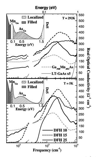
FIG. 6. The effective conductivity of a doped layer  $[\sigma_1^{el}(\omega)]$  extracted using the EMT analysis of raw data as described in the text. The top panel shows the result at 292 K and in the bottom panel 5 K results are plotted. Also shown are  $\sigma_1(\omega)$  for Ga<sub>0.948</sub>Mn<sub>0.052</sub>As and  $\sigma_1(\omega) \times 5$  for LT-GaAs.
