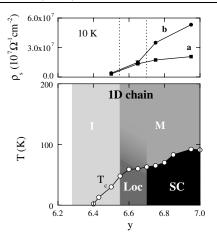
FIG. 3. Top panel: the doping dependence of the superfluid density  $\rho_s$  at y = 6.50-6.95 [5] separately for *a*-axis and *b*-axis data. Bottom panel: phase diagram displaying characteristic regimes in the response of the Cu-O chains. Here I stands for insulating, LOC for localized metal, M for Drude metal, and SC for superconducting.
